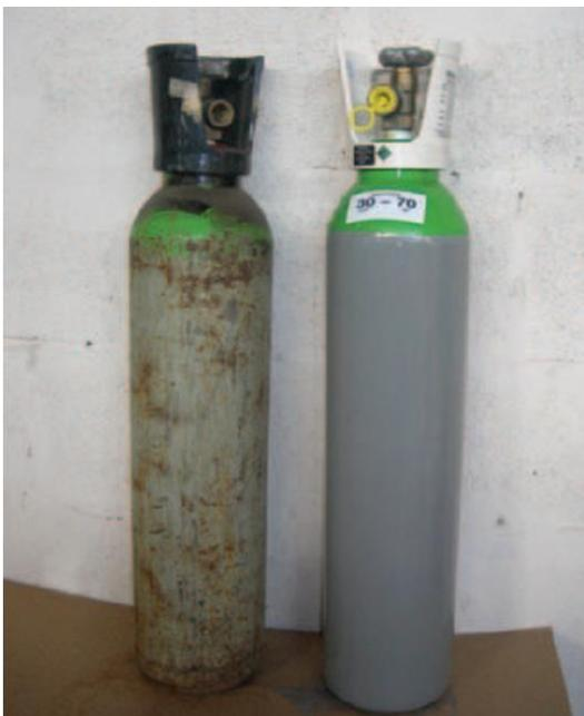
Such cylinders have violently ruptured in cellars, causing immense damage and injury. Short of rupture, licensees should realise that even a slow leakage of a non-breathable gas within the confined space of a cellar could lead to a very hazardous atmosphere. Carbon Dioxide and Nitrogen have no odour and people have died in such atmospheres.
